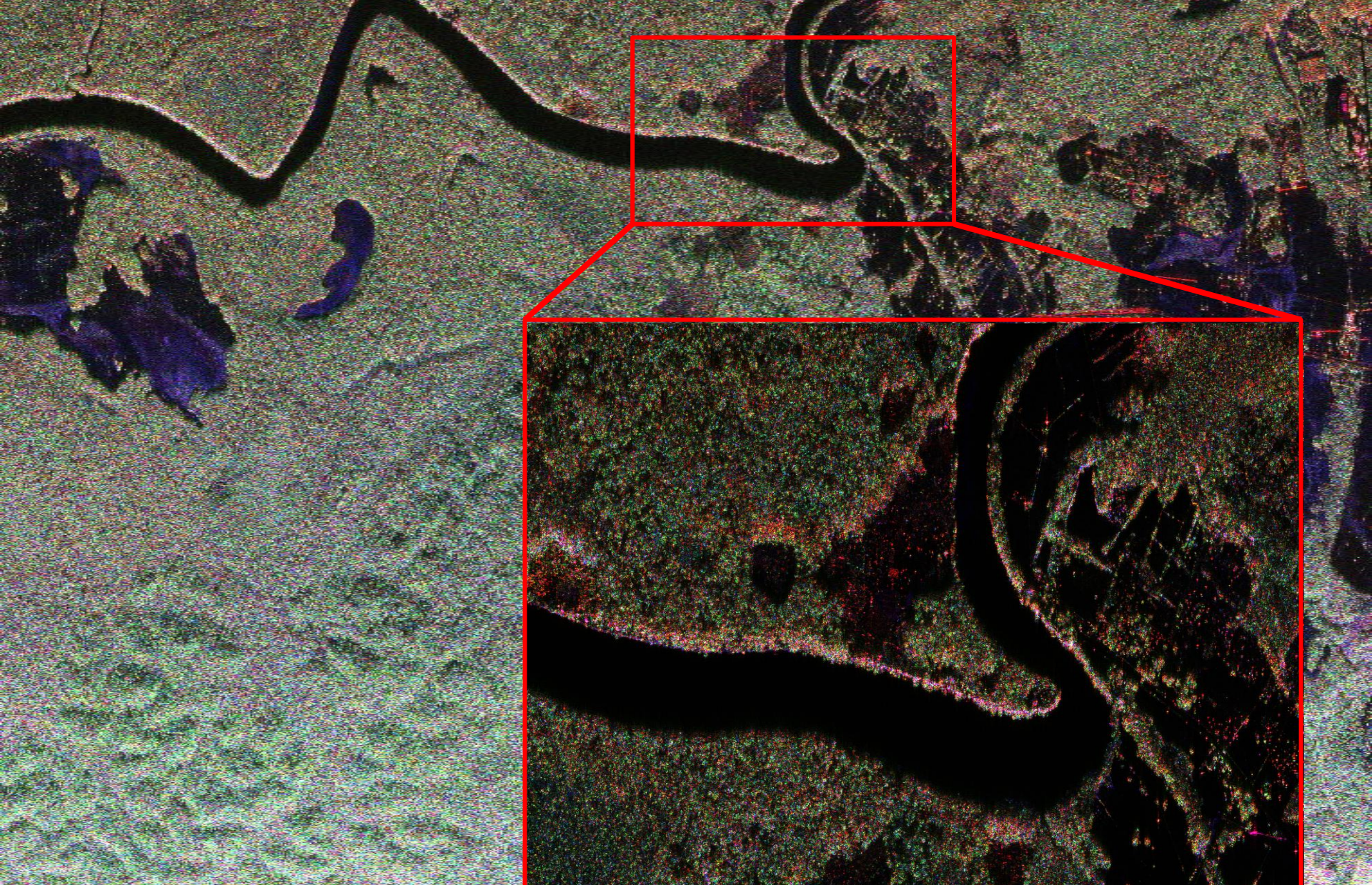
P-Band airborne SAR image of the tropics with a resolution of 1 m. This picture is obtained as a color-composite representation of the magnitudes of three images acquired using different wave polarizations at Tx and Rx. Data gathered by ONERA during the ESA campaign TropiSAR, 2009.
